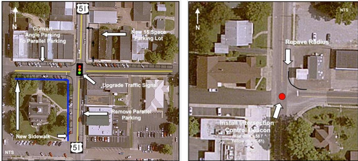
**FIGURE 7: IMPROVEMENTS AT CLAY ST (LEFT) AND MAYFIELD RD (RIGHT)**
