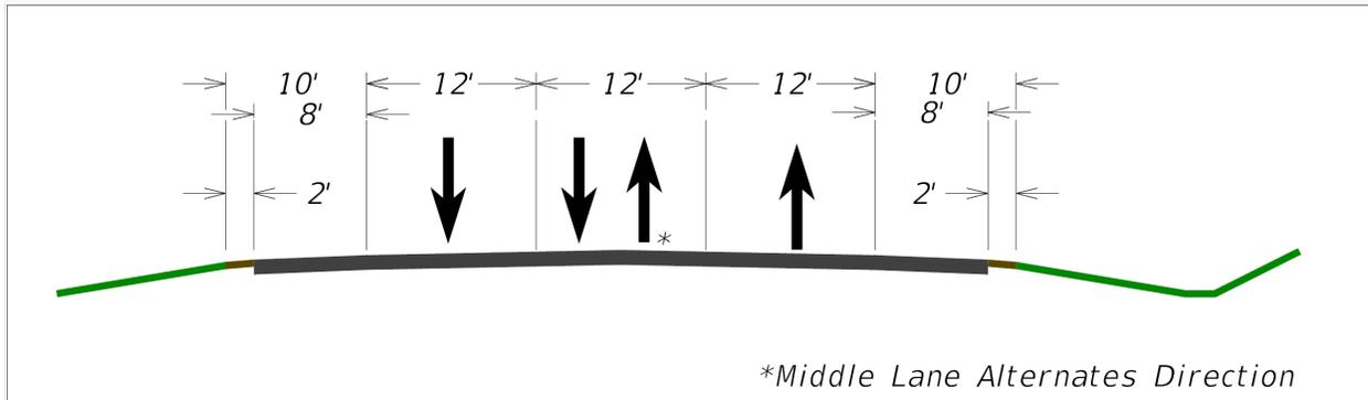
**FIGURE 36: PROPOSED TYPICAL SECTION FOR 2+1 WIDENING**
